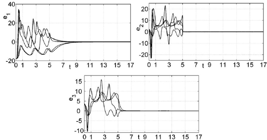
**Fig. 3. Evolution of the dynamic errors for controlled PMSM system considering uncertain parameters**
