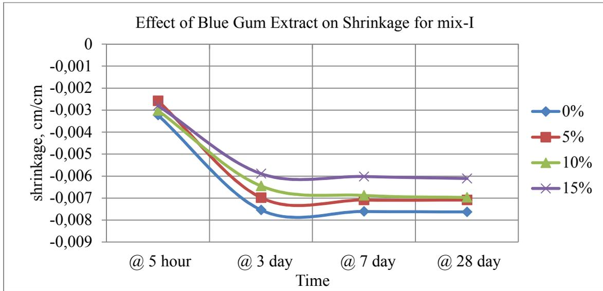
Figure 2: Shrinkage through time for different dosage for controlled from direct heat from the sun
