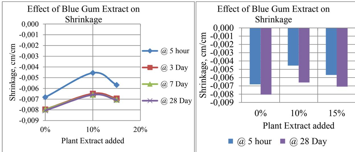
Figure 3: The Effect on shrinkage for exposed to direct heat from the sun
