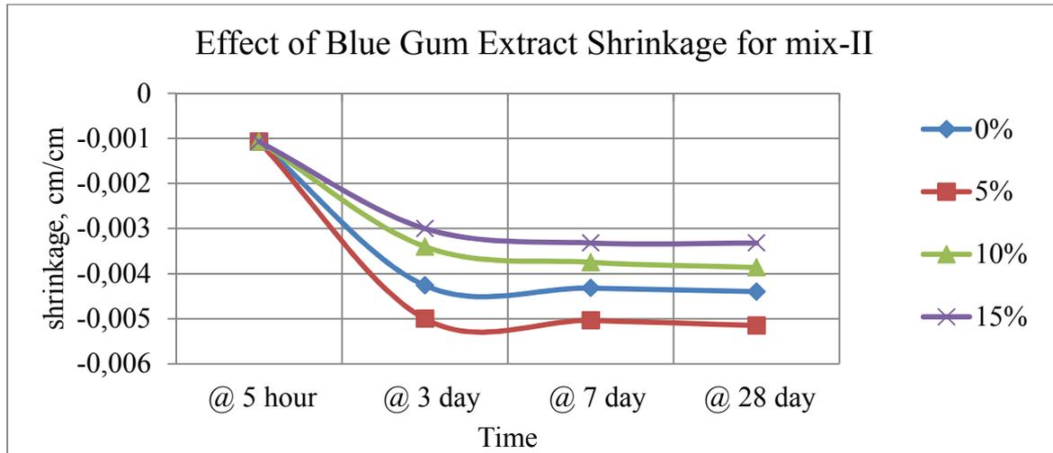
Figure 6: Shrinkage through time for mix-II controlled from direct heat from sun
