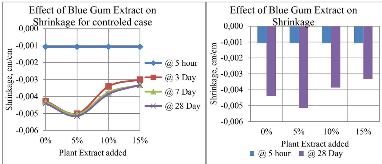
Figure 1: The Effect of Blue Gum Extract on shrinkage for controlled case for slab exposed to direct heat from the sun
