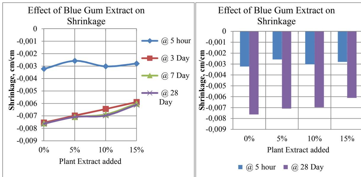
Figure 1: The Effect blue gum extract on shrinkage for controlled from direct heat from the sun
