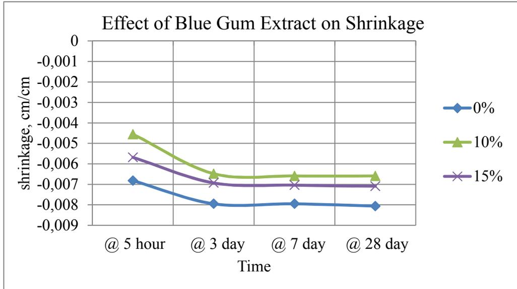
Figure 4: Shrinkage through time for different dosage for slab exposed to direct heat from the sun
