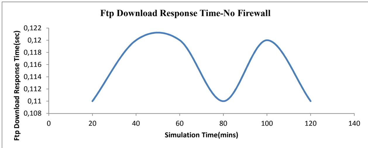
*Fig.12: Ftp Download Response Time – No Firewall Scenario*
