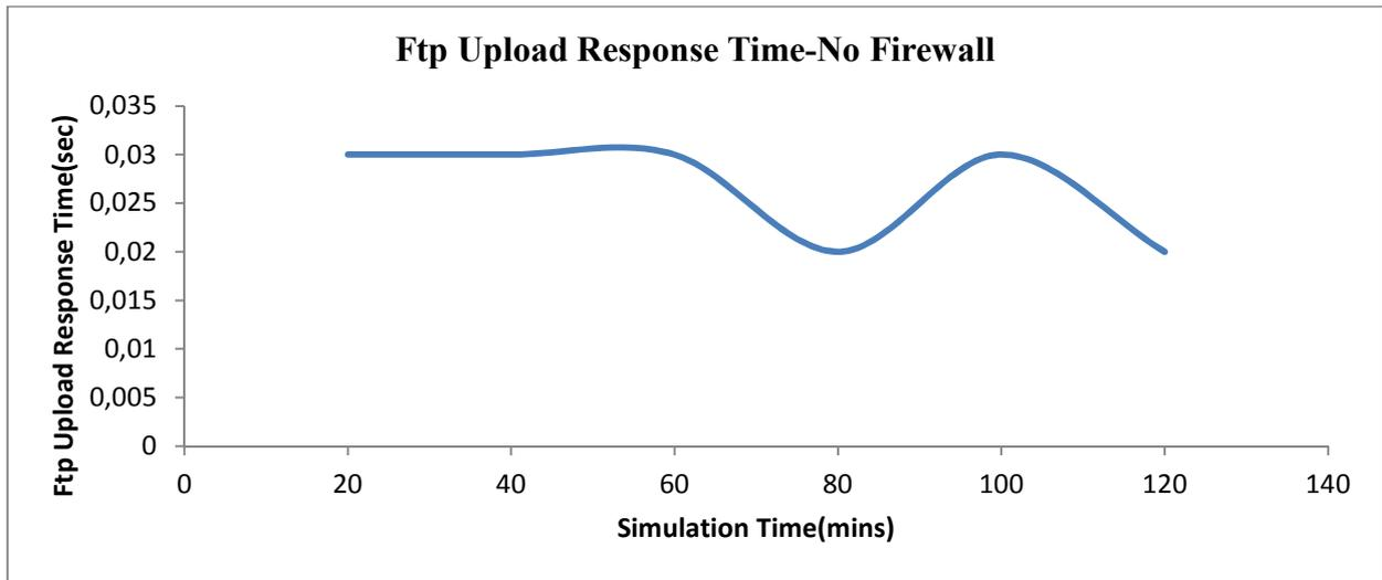
*Fig.16: ftp upload response time – No firewall scenario*
