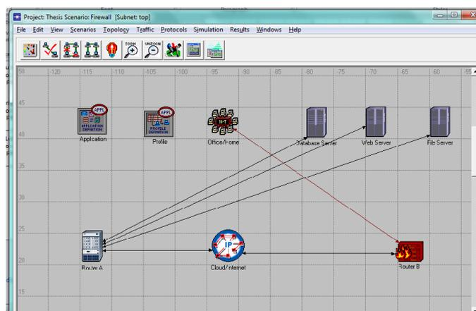
Fig.2 Firewall Scenario setup Network Layout (M. Asante ,F.K. Agbenyegah,A. Osei-Owusu (2014))
