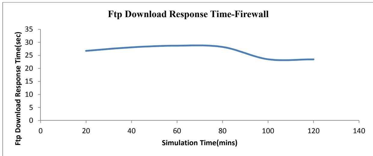
*Fig13: Ftp Download Response Time – Firewall Scenario*
