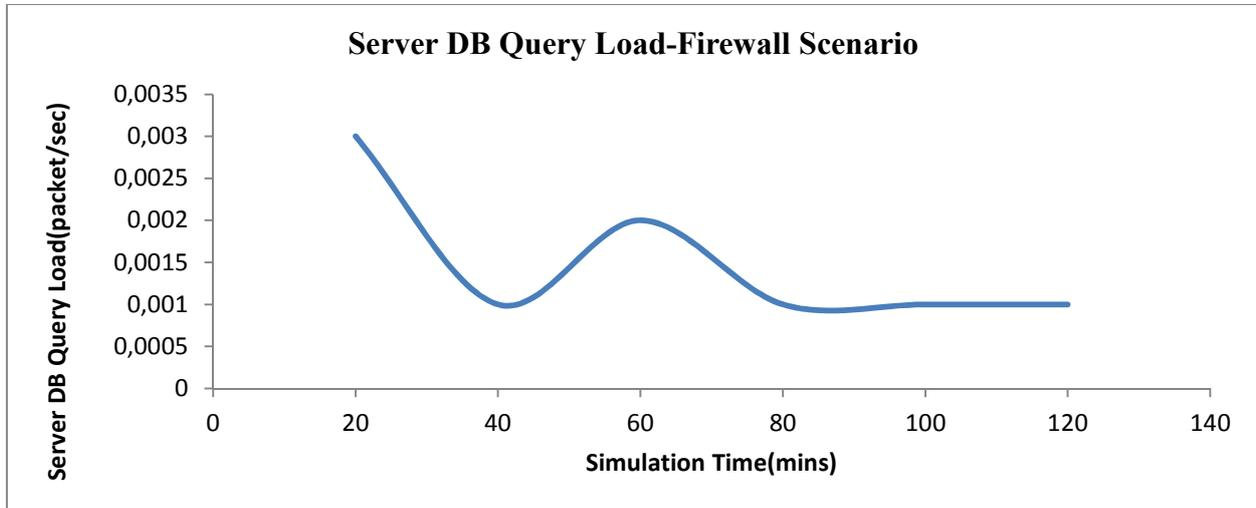
*Fig. 9: Server Database Query Load - Firewall Scenario*
