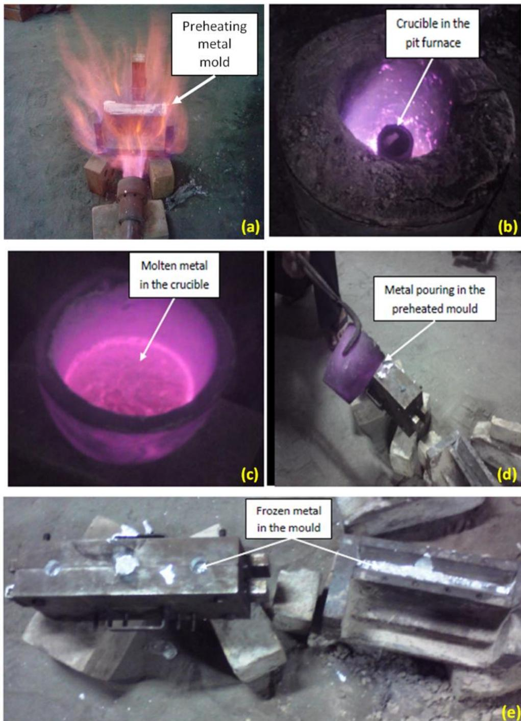
Fig. 2. Preparation of Zn-Ni Solder alloys (Casting Route)
