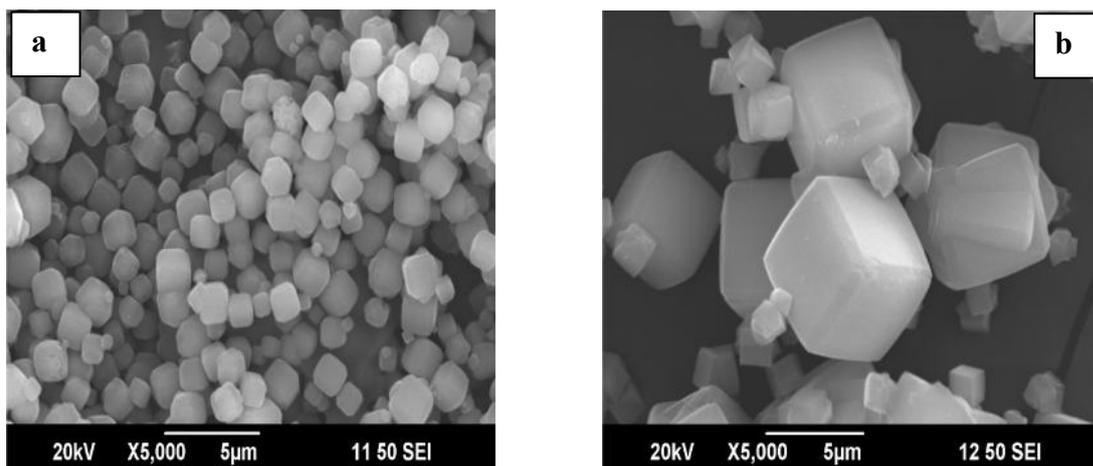
Figure.3. SEM images of (a) WSZ and (b) WSZ<sub>m</sub>
