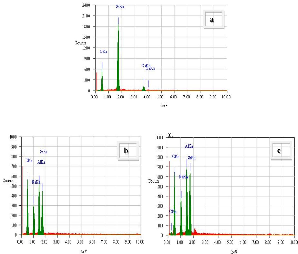
Figure.2. EDX analysis of (a) Wheat ash (b) WSZ and (c) WSZ<sub>m</sub>
