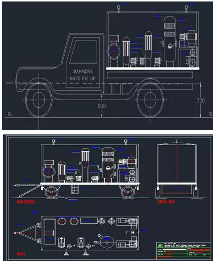
Space available to use on Mahindra Bolero is measured and accordingly it is designed by using software of Auto CAD.
