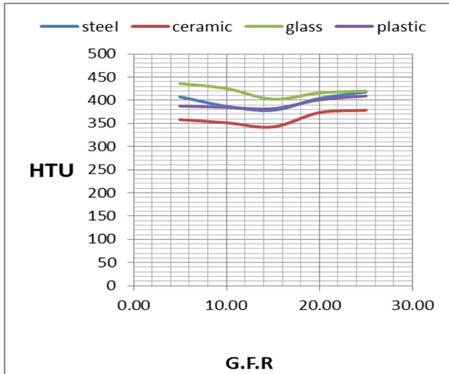
Figure 2 straight line equations and graphical trends of packing studied (O<sub>2</sub> absorption)
