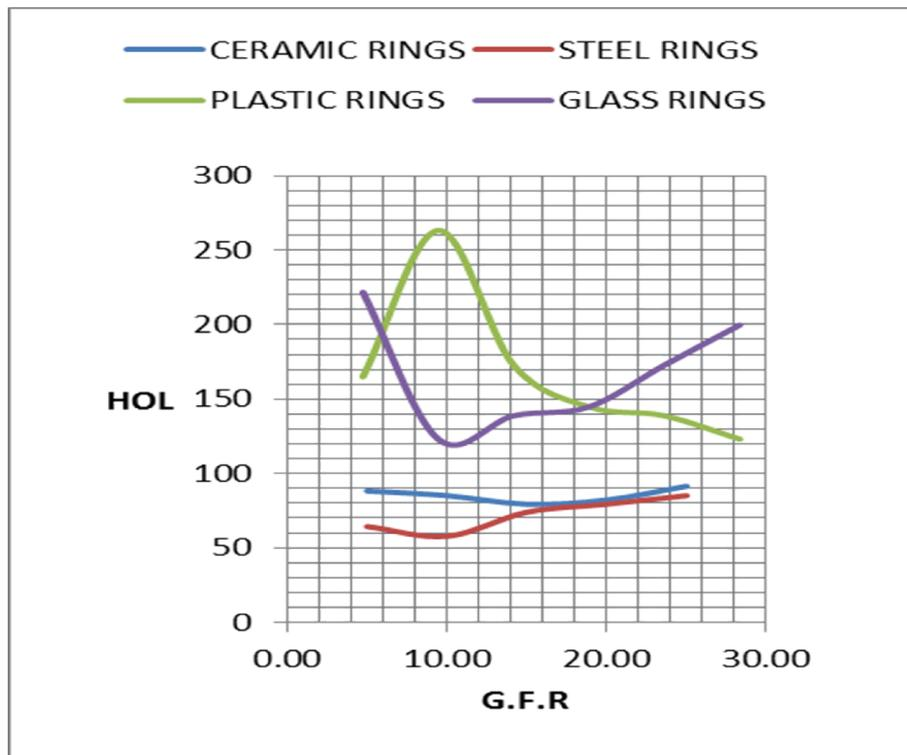
Figure 1 straight line equations and graphical trends of packing studied (CO<sub>2</sub> absorption)
