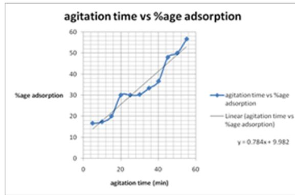
Figure 2 effect of agitation time on %age adsorption for congo red
