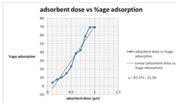
Figure 4 effect of adsorbent dose on %age adsorption for congo red
