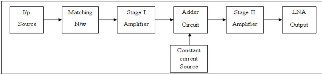
Fig. 3. Block Diagram of Proposed design
