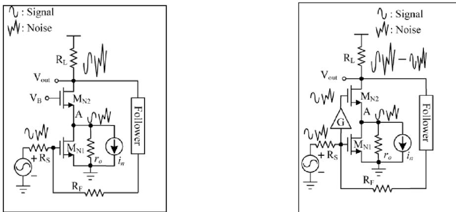
Fig. 1. Conventional resistive negative feedback. Fig. 2. Resistive feedback with noise cancellation technique
