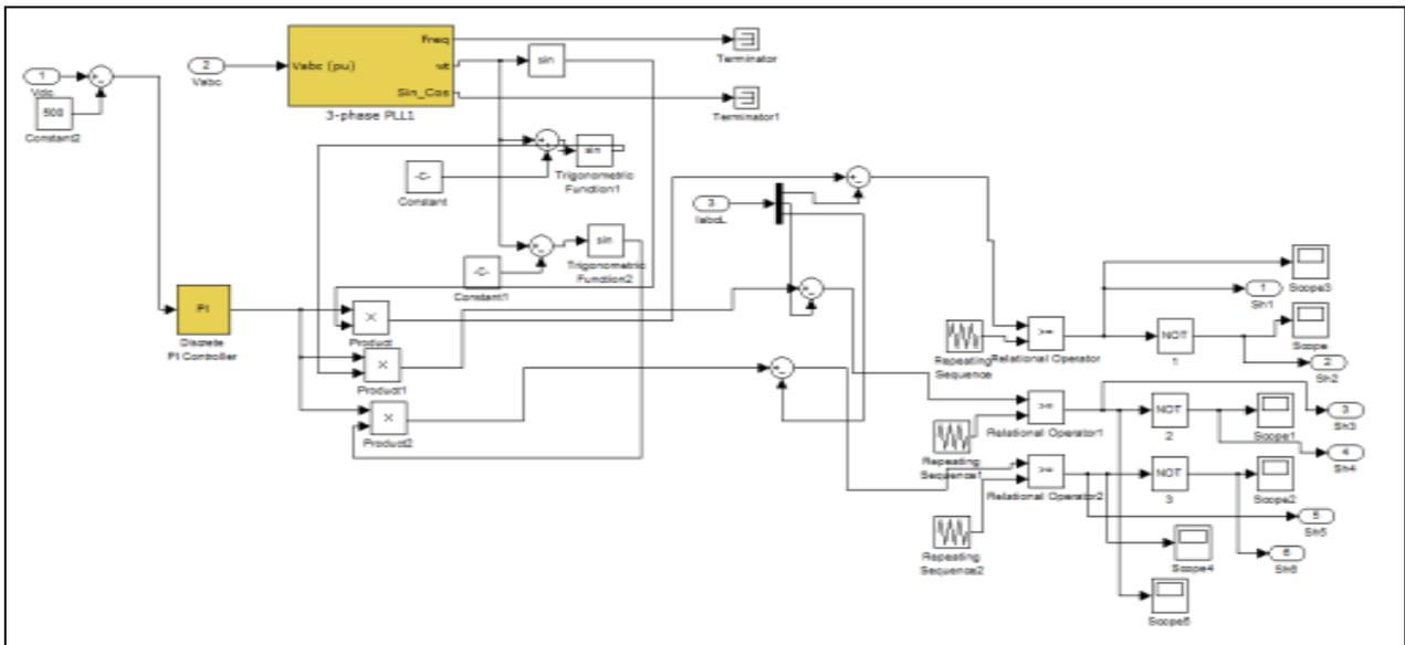
Fig 4 Simulink model of SPWM
