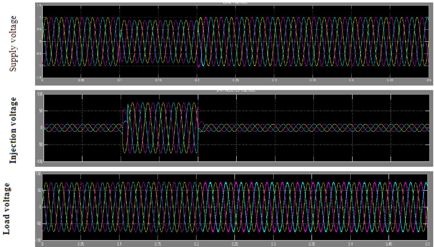
Fig. 6 DVR response to balanced voltage Sag
