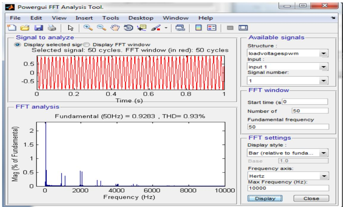
Fig.7 waveforms of showing the FFT analysis of load voltage of spwm
