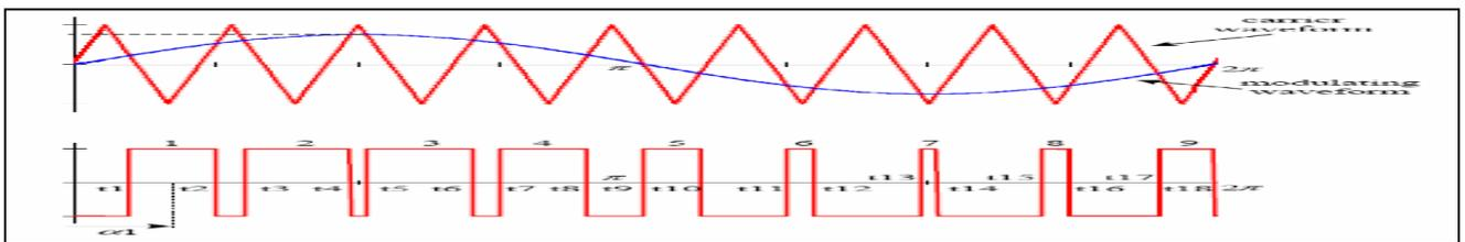
Fig. 3. Sinusoidal pulse-width modulation
