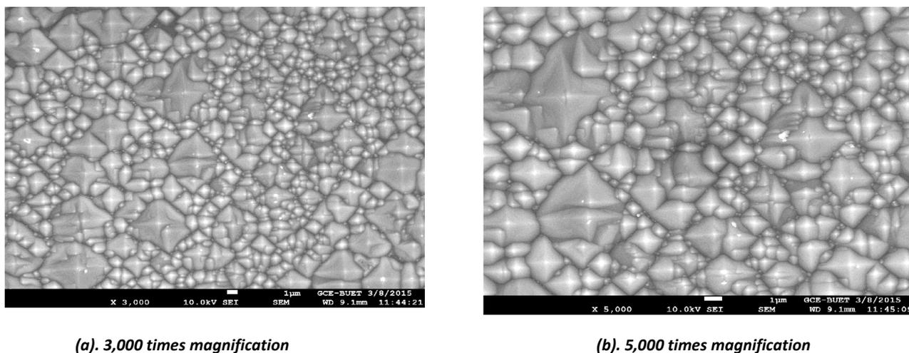
Fig.4. SEM image of textured silicon wafer
