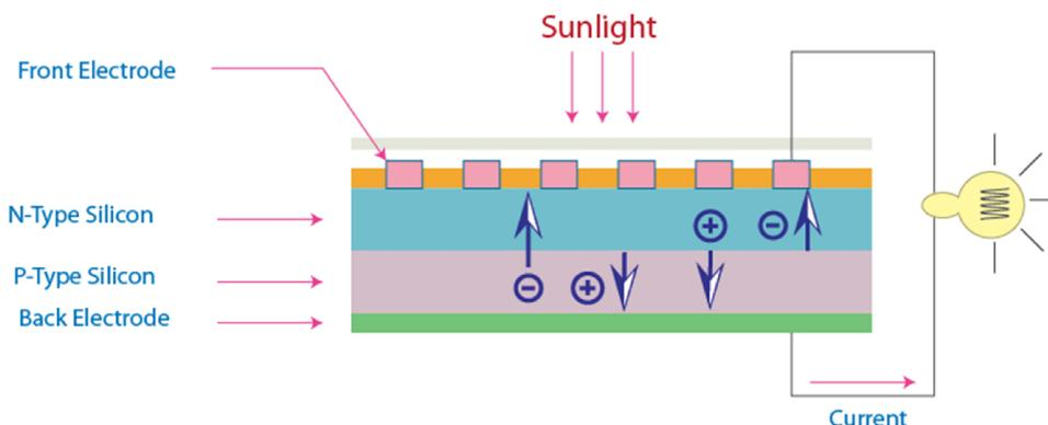
Fig.1. Solar Cell Operation
