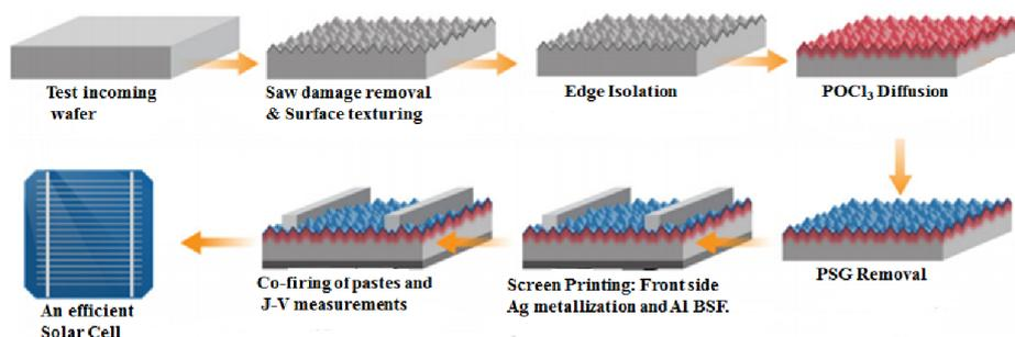
Fig.2. Steps of solar cell fabrication process.
