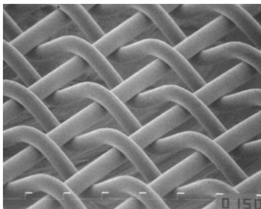
Fig.7. a) Microscopic image of the screen
