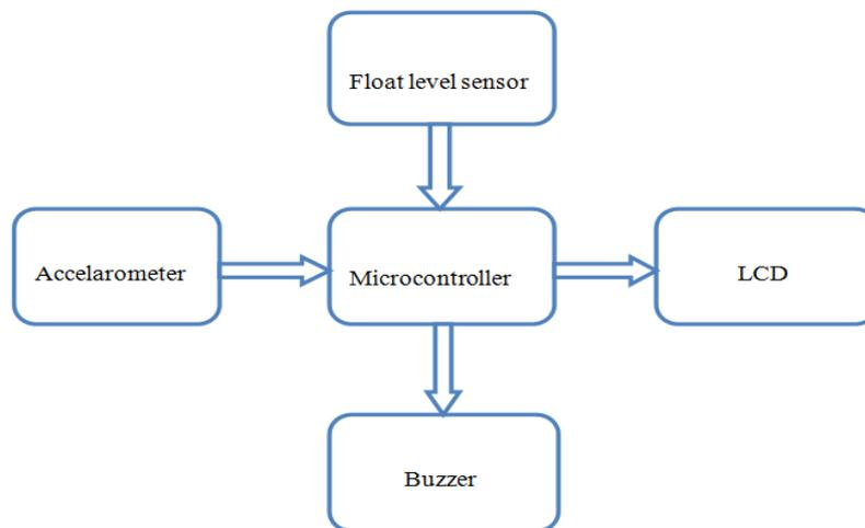
Fig. 7. Block Diagram of Earthquake Detection Process
