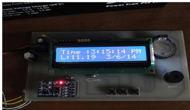
**Fig. 11. Earthquake Detected by the Accelerometer**
