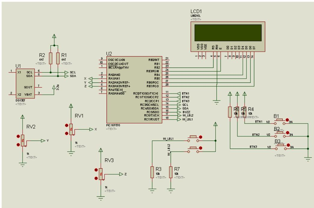
Fig. 9. Schematic Circuit Diagram of Tsunami Detector
