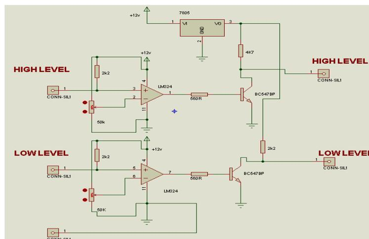
Fig. 8. Water Level Sensor Diagram
