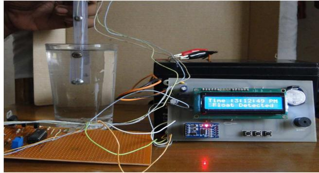
**Fig. 12. Float Detected By The Water Level Sensor**
