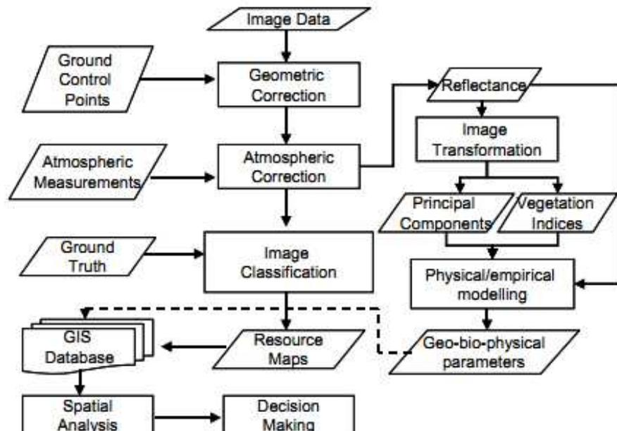
Figure 4. A schematic diagram of general image processing procedures, (Source: Campbell, 2007)
