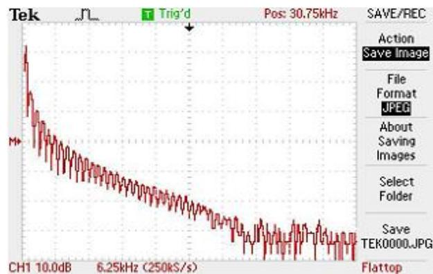
**Fig. 8. Fast Fourier transform of the VSC output with SPWM technique**
