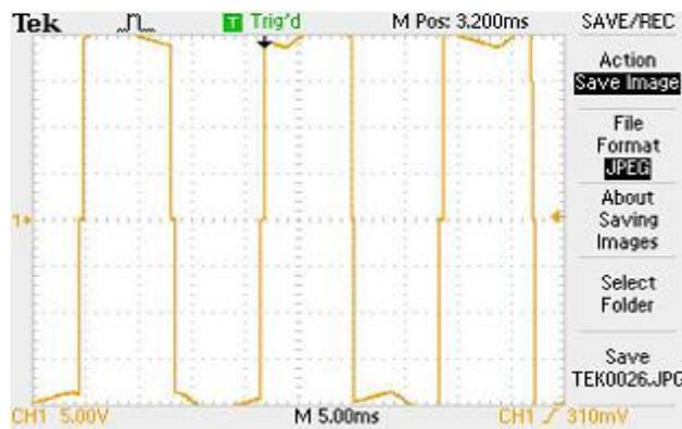
**Fig. 7. Output at Inverted Sine carrier wave**
