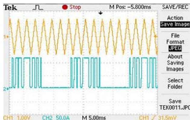
**Fig. 5. Pulses generated using ISPWM Technique**
