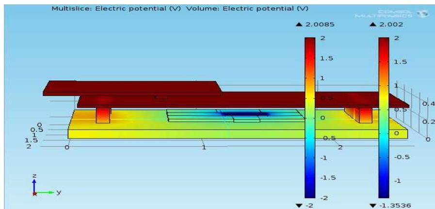
Fig-3 shows potential applied between ribbon actuator and one of the electrodes
