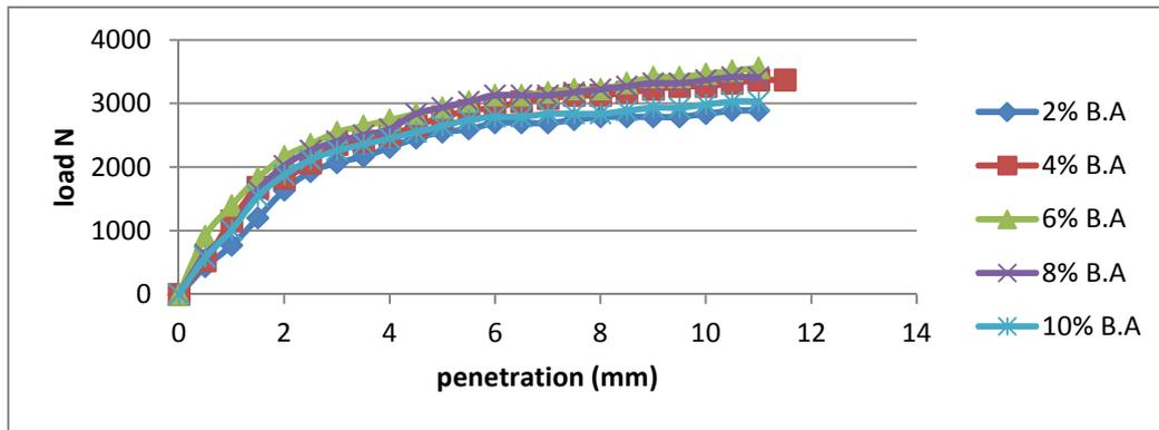
Fig. 2. CBR plot for soil with bagasse ash
