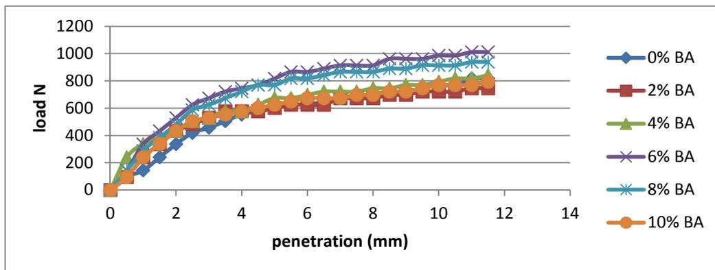
Fig. 4. CBR plot for soil with bagasse ash and double layer geogrid
