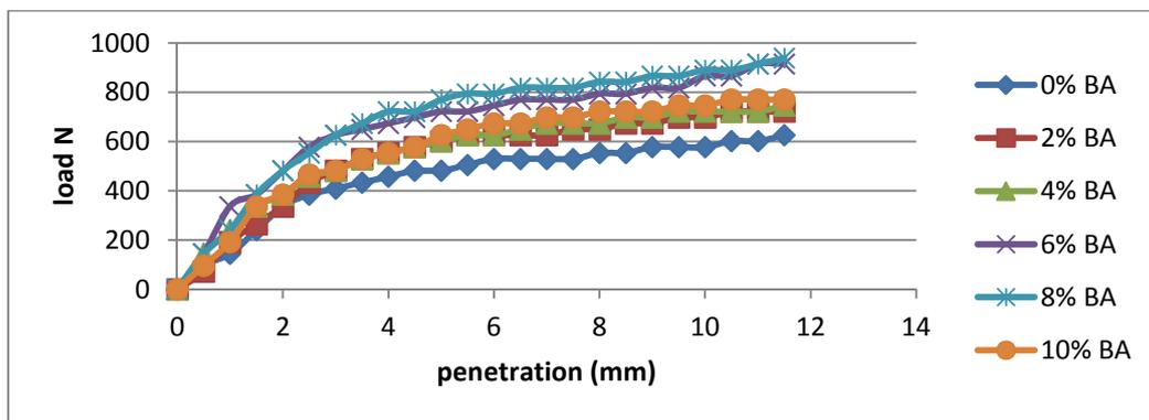
Fig. 3. CBR plot for soil with bagasse ash and single layer geogrid
