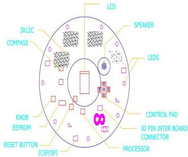
**Figure2 Robot controller board**
