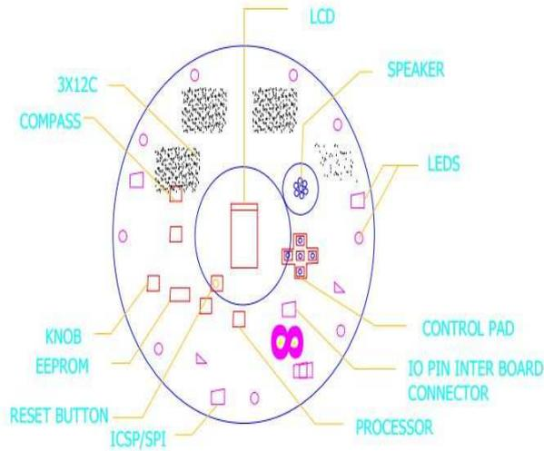
**Figure2 Robot controller board**
