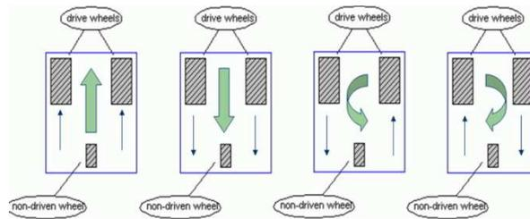
**Figure3 Robot wheeling**
