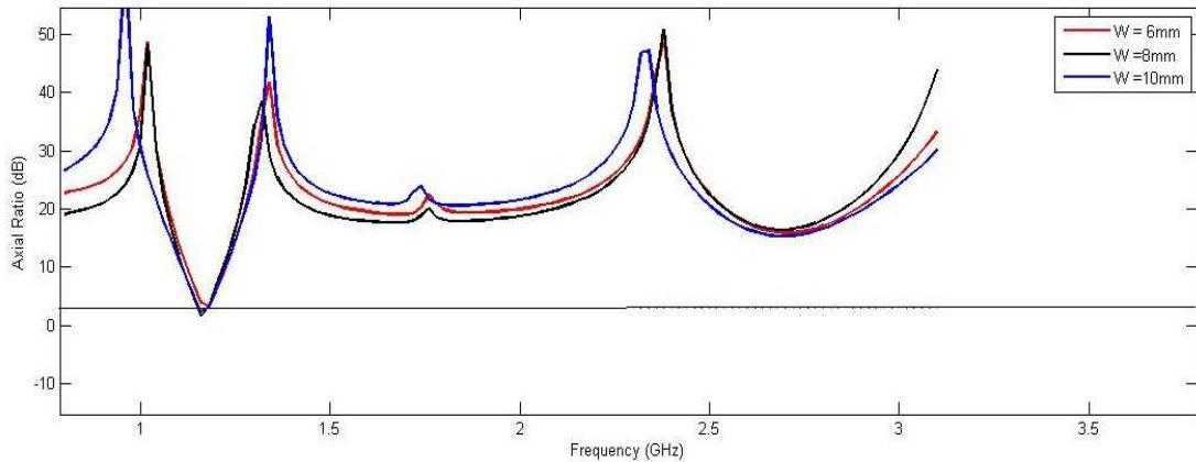
*Fig.4. Simulated axial ratio for different stub width*
