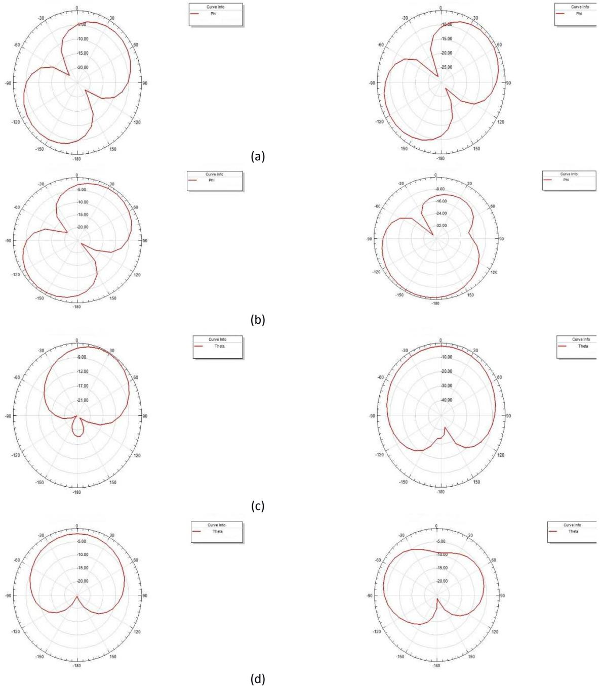
**Fig.6. Measured radiation pattern for the proposed antenna**
