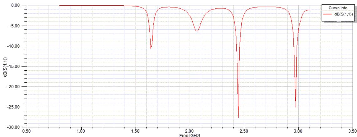
Fig.3. Simulated return loss for proposed antenna
