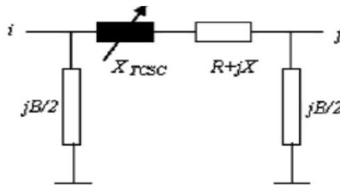
Fig.2 Single line diagram of power flow control with TCSC
