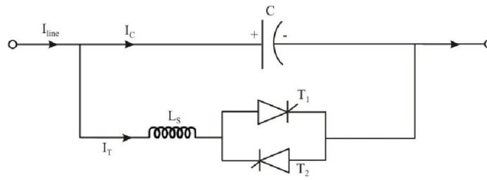
Fig 1. Basic structure of Thyristor controlled-series capacitor
