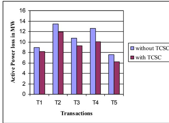
Fig 5. Active Power Loss (bilateral Transaction) for IEEE 30 bus system Base case
