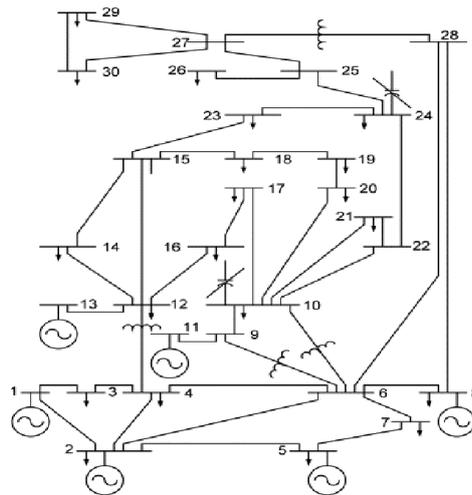
Fig 3. Single line diagram of the modified IEEE 30-bus system
