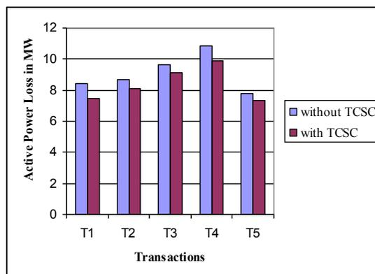
Fig 7. Active Power Loss (bilateral Transaction) for IEEE 30 bus system with line outage of 9-10
