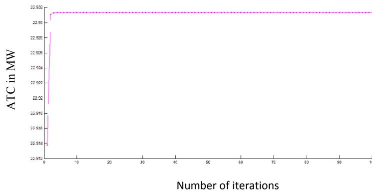
Fig 6. PSO convergence curve for multilateral transactions with TCSC under normal operating condition
