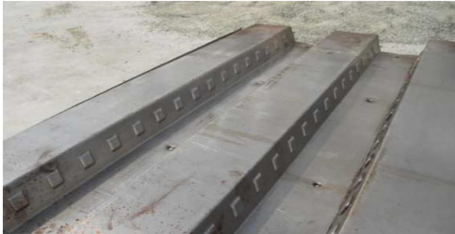
*Fig.2. Rectangular Dishing Type Embossment*
