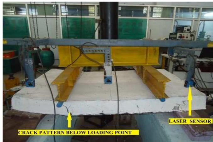
Fig.11. Crack pattern of composite slab
