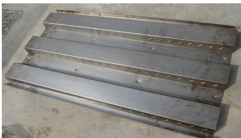
Fig.6. Inclined Penetrated Embossment
