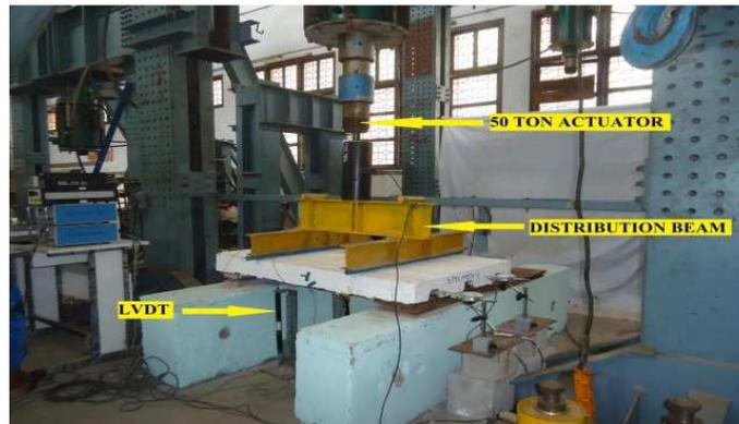
Fig.9. Experimental setup of loading frame
