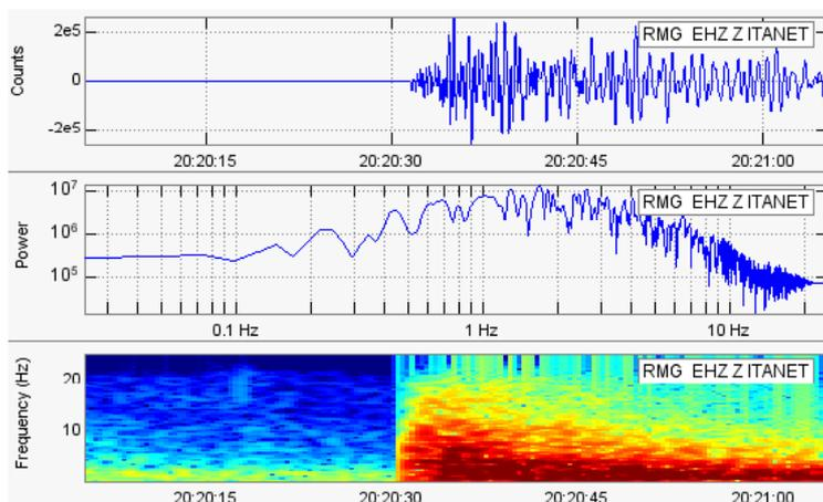
Fig. 7. Waveform, spectrogram and spectrum of a typical Hybrid event recored at Katala station renamed RMG after the deployment of the broadband 40s. the Frequency Contant reaches values about 8Hz.
