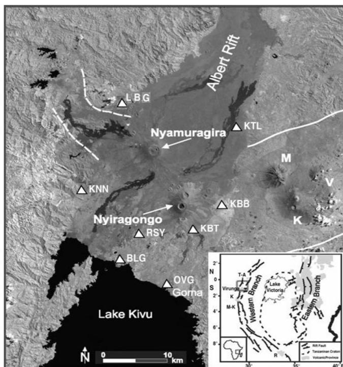
Fig. 4. Seismic network of the Goma Volcano Observatory. Seismic stations are marked by white triangles (Goma-OVG, Kunene-KNN, Rusayo-RSY, Bulengo-BLG, Kibumba-KBB, Kibati-KBT, Katale-KTL, Luboga-LBG). Volcanoes: K-Karisimbi, M-Mikento, V-Visoke. Inset shows eastern and western branches of East African Rift System. Volcanic provinces in the western branch: T-A-Toro-Ankole, K-Kivu, M-K-Mwenga-Kamituga, R-Rungwe. Modified after References [30] and [31].
