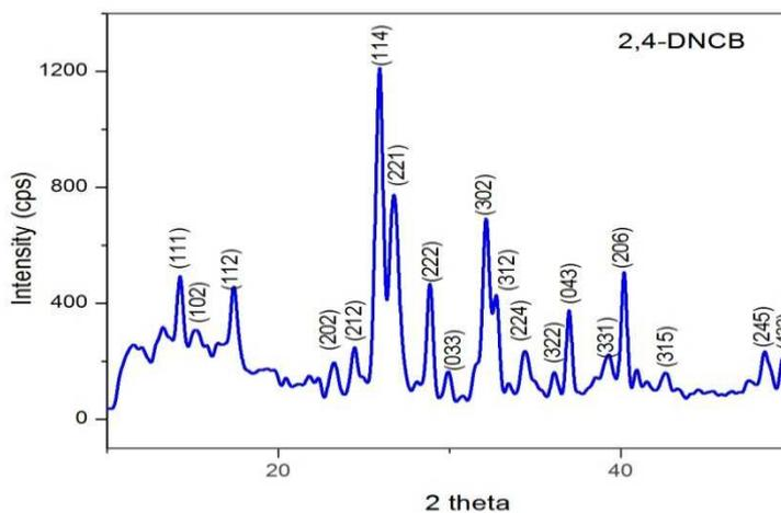
Fig. 4. Powder XRD spectrum of DNCB crystal
