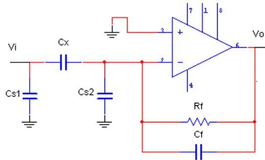
*Fig. 2. AC-based capacitance measuring circuit with stray capacitances*
