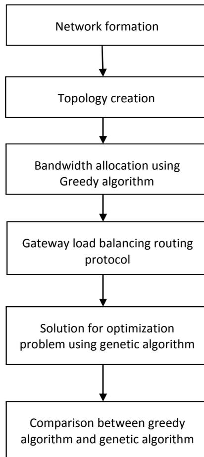
**Fig. 1. system architecture**
