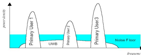
Fig 4 Illustration of Cognitive Radio Underlay Concept
