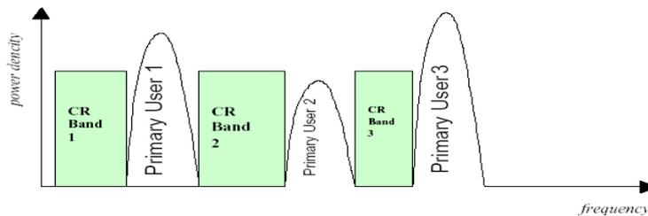
Fig 3 Illustration of Cognitive Radio Overlay Concept
