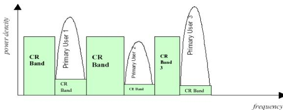
Fig 5 Illustration of Cognitive Radio Hybrid Overlay/Underlay Concept
