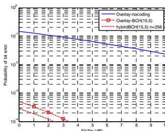
Fig 9 Performance of Hybrid overlay/underlay waveform using BCH codes in Frequency selective Fading channel
