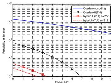
Fig8 Performance of Hybrid overlay/underlay waveform using Hamming codes in Frequency selective Fading channel
