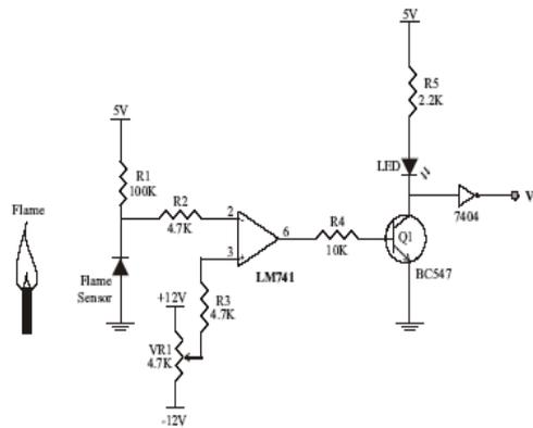
Fig.7 Flame sensor circuit
