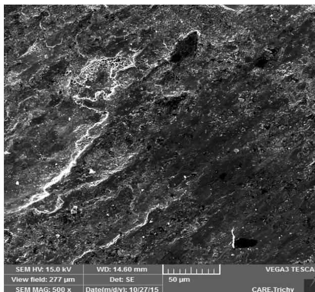
*Fig. 6 (c) SEM image on worn-out surfaces of Fe-1%C*
