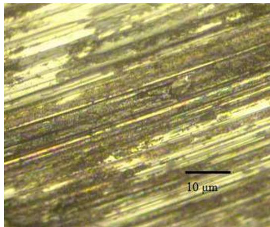
*Fig. 6 (b) maximum wear worn-out surfaces of Fe-1%C-1%Ti*
