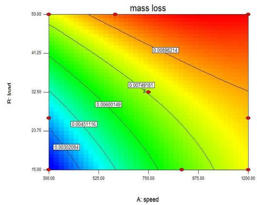
Fig.2 (b) 2D- contour surface plot graph for Fe-1%C
