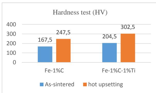
Fig. 1 Hardness test for both as-sintered and hot upsetting specimens
