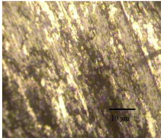
*Fig. 6 (a) maximum wear on worn-out surfaces of Fe-1%C*
