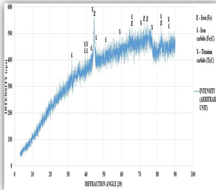
Fig.4 (b) XRD peak analysis on wear debris of Fe-1%C-1%Ti
