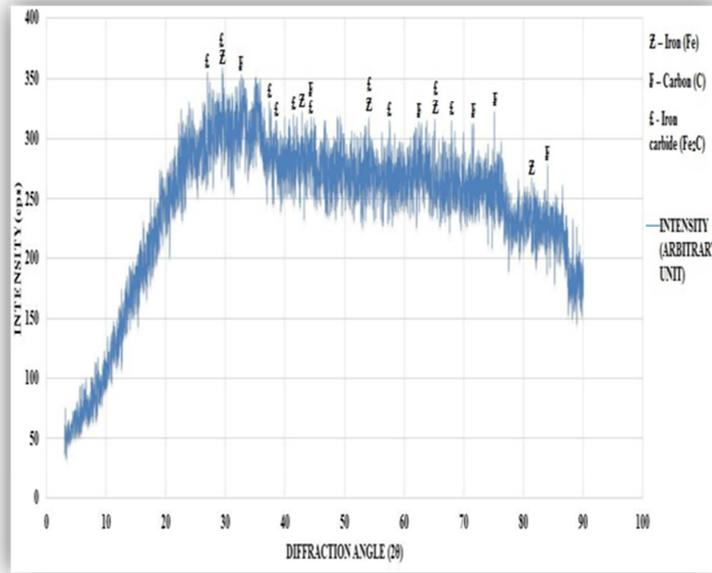
Fig.4 (a) XRD peak analysis on wear debris of Fe-1%C
