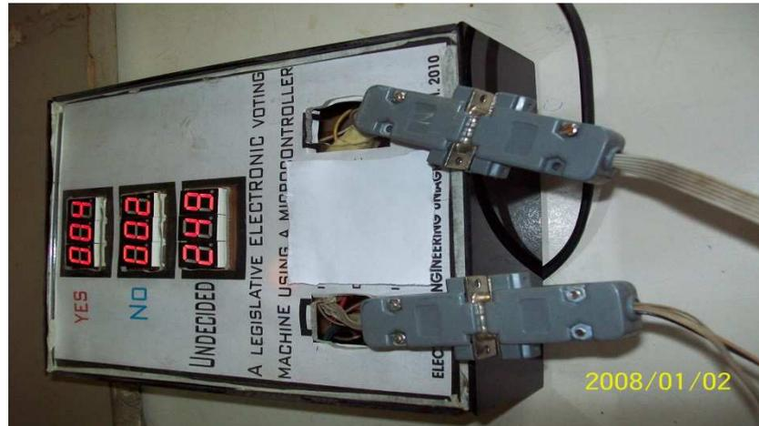
Fig. 10. A View of the Legislative Voting System Showing Only the Display Unit
