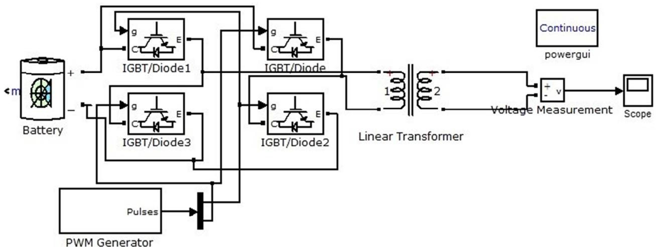
Figure 5: Simulink Model for DC-AC Bridge Inverter
