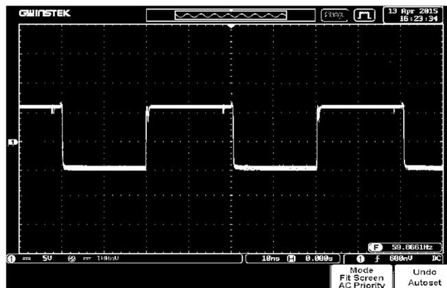
Figure 4: Hardware DC-AC Inverter Bridge output at 60 Hz
