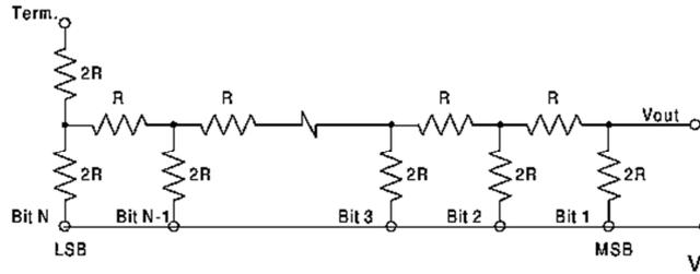
Figure 8: R/2R ladder network for DAC [15, 17]
