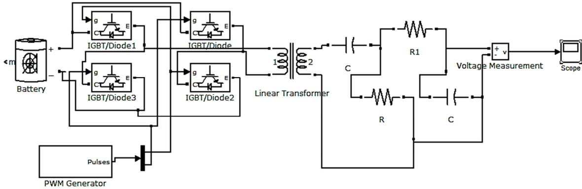
Figure 11: DC-AC Inverter with Band Pass Filter
