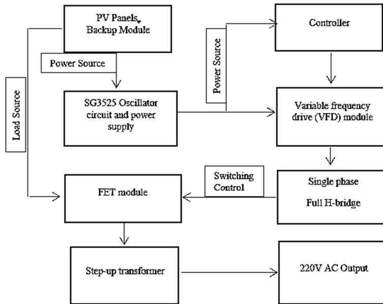
Figure 6: Process flow of DC-AC Bridge Inverter [4]
