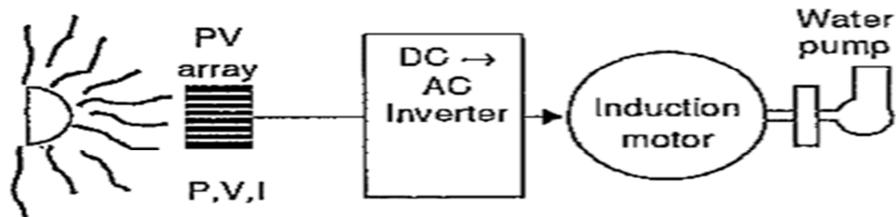
Figure 1: Process flow of the System [2]
