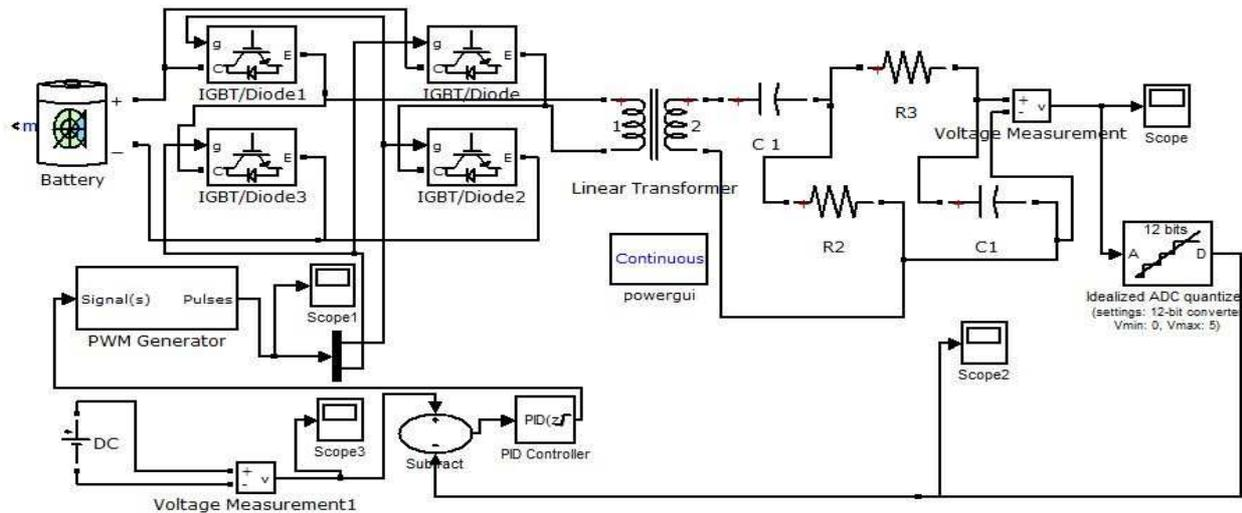
Figure 18: DC to AC Inverter with PID Voltage Control
