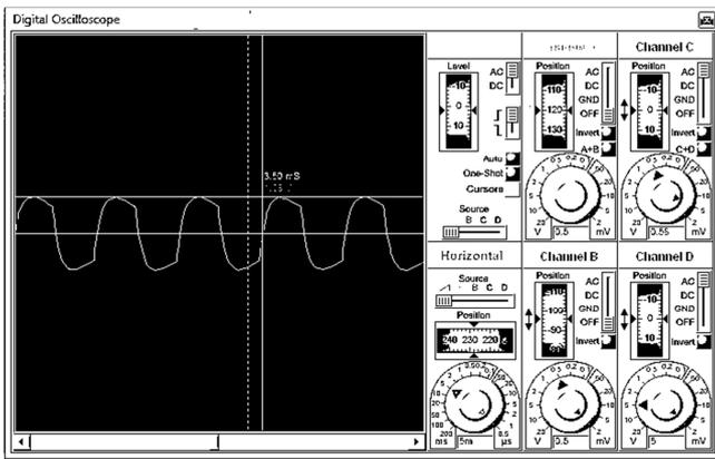
Figure 12: Output with Band Pass Filter on Proteus
