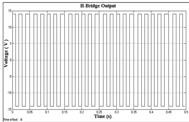
Figure 3: Simulink DC-AC Inverter Bridge output at 60 Hz
