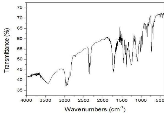
**Fig. 6. Spectra of 30 wt% Fiber Reinforced PP Composite**
