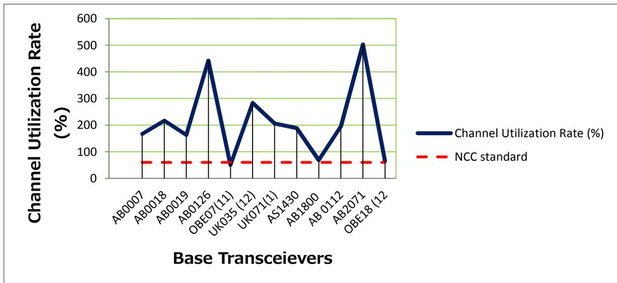
Fig 3 Comparing Channel Utilization Rate of the Network with the NCC Standard
