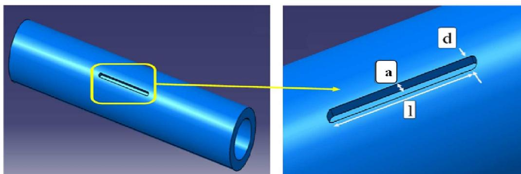
**Fig. 2. Grooves dimensions**
