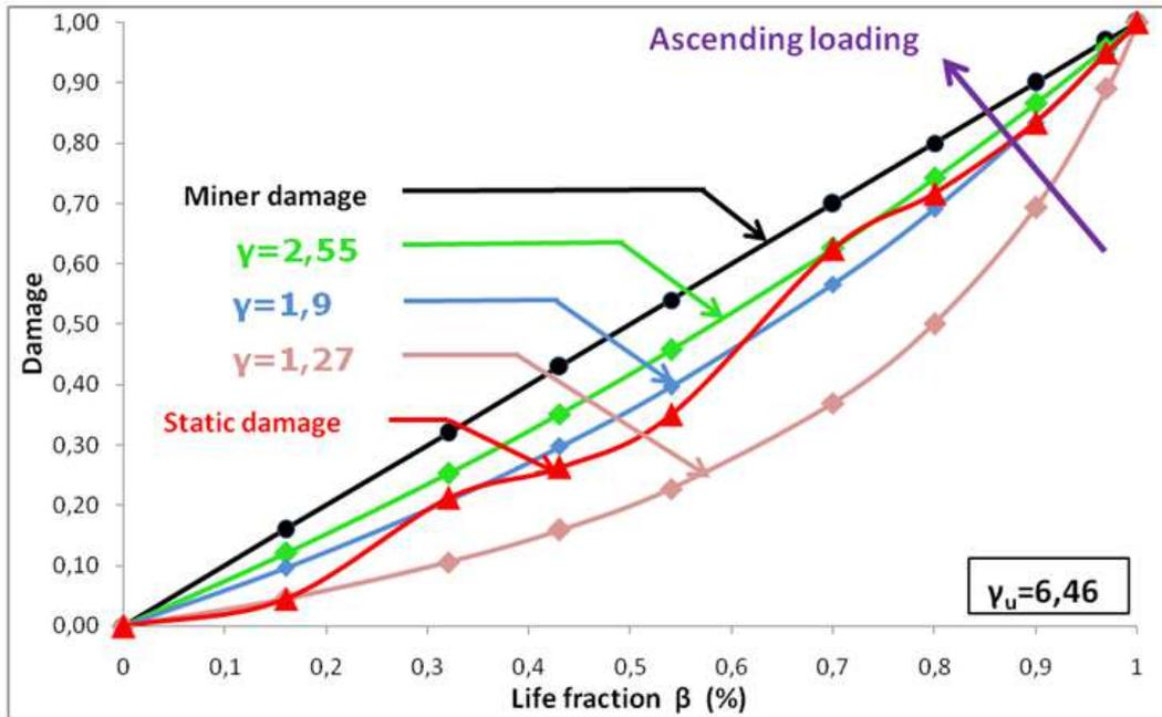
Fig. 8. Static, unified and Miner damages comparison
