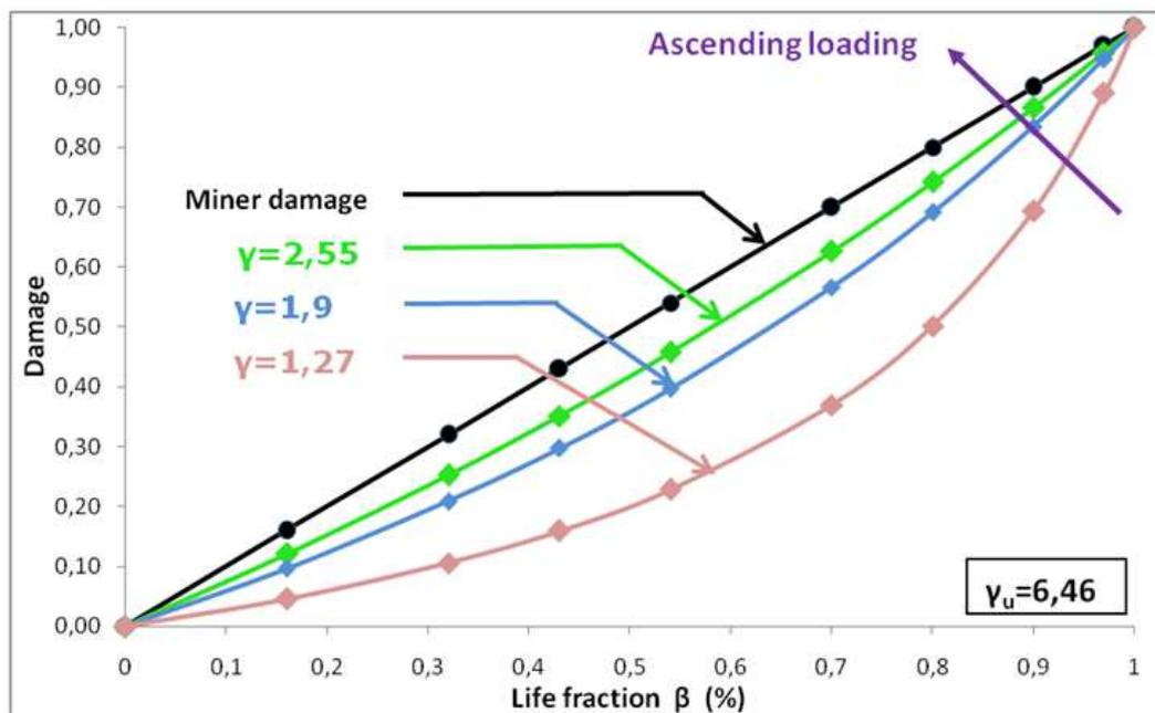
Fig. 7. Unified damage variation in function of the life fraction
