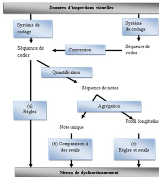
*Figure1. Steps and sub-problems for the assessment of an anomaly indicator from the visual inspection data of a section*
