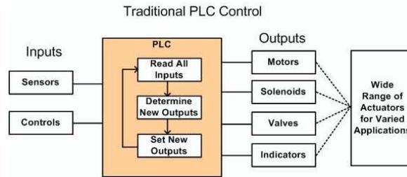
In this application, it controls through analog/digital inputs and outputs by varying the speed through VFD of an induction motor. Also the PLC reads the input and control the outputs according to the PLC program. This PLC is a Delta type of ISP software where the link is made to the system through RS232 cable. It has an advantage that the initial configuration can be expanded for the other applications as machine systems and computer related linking
