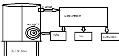
*Fig.2. Block diagram*
