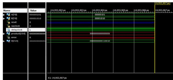
Fig. 8. output for 8 bit vedic multiplier with razor
