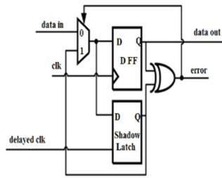
Fig. 4. Diagram for Razor Flip Flop
