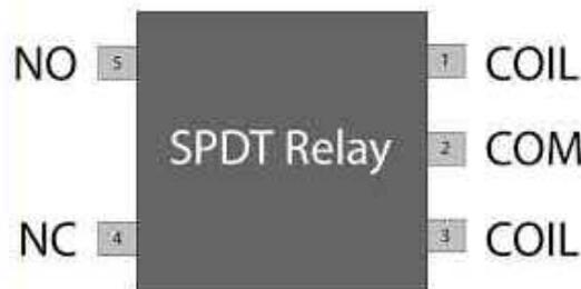
*Fig 6. Pin diagram of relay*
