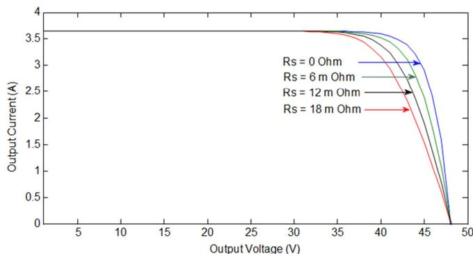
Figure 4. Effect of series resistance on the I-V characteristic.
