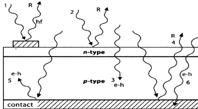
Figure 1. photovoltaic cell
