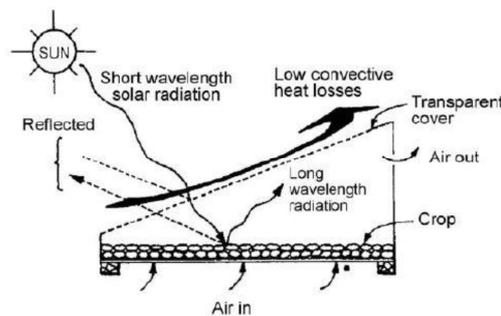
*Fig 3.1: Working of Cabinet type of dryer*
