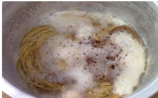
**Fig3.14 Reaction of fibre with NaOH**
