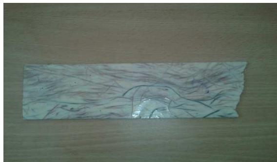
**Fig 3.15 Final composite for tensile testing**
