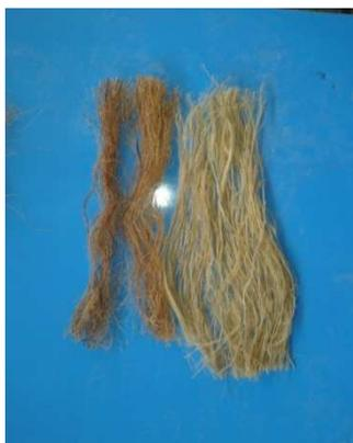
*Fig. 3.10 Bamboo and Banana Fibres*
