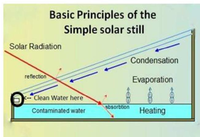
Water to be cleaned is poured into the still to fill at certain amount of the basin. The glass cover allows the solar radiation to pass through and it reaches the bottom of the still which is mostly absorbed by the base because the surface is coated with black colour material to increase the sun heat absorption. The water begins to heat up and the moisture content of the air trapped between the water surface and the glass cover. Due to heating water gets evaporated from the basin and
