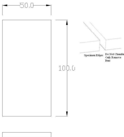
Figure 2: Workpiece Dimensions
