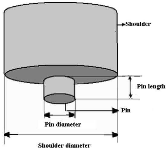
Figure 4: Tool Geometry
