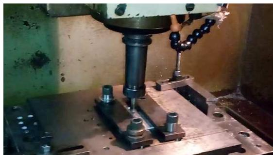
Fig.1. Friction Stir Welding Experimental Setup
