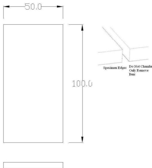
Figure 2: Workpiece Dimensions
