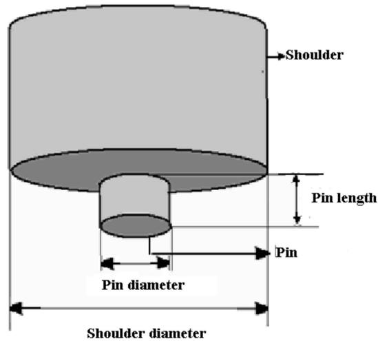
Figure 4: Tool Geometry
