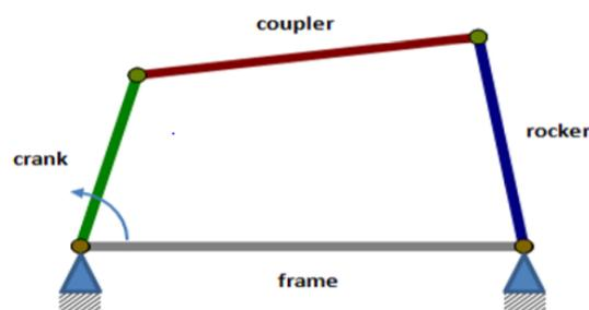
Fig.1.1 Four bar linkage
