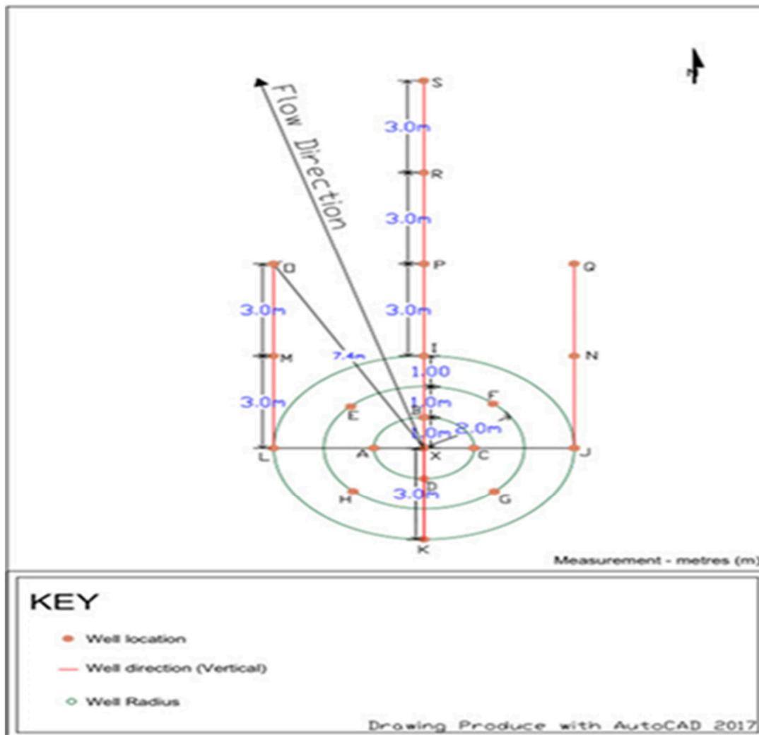
Fig. 1. Schematic Layout of tracer test field design
