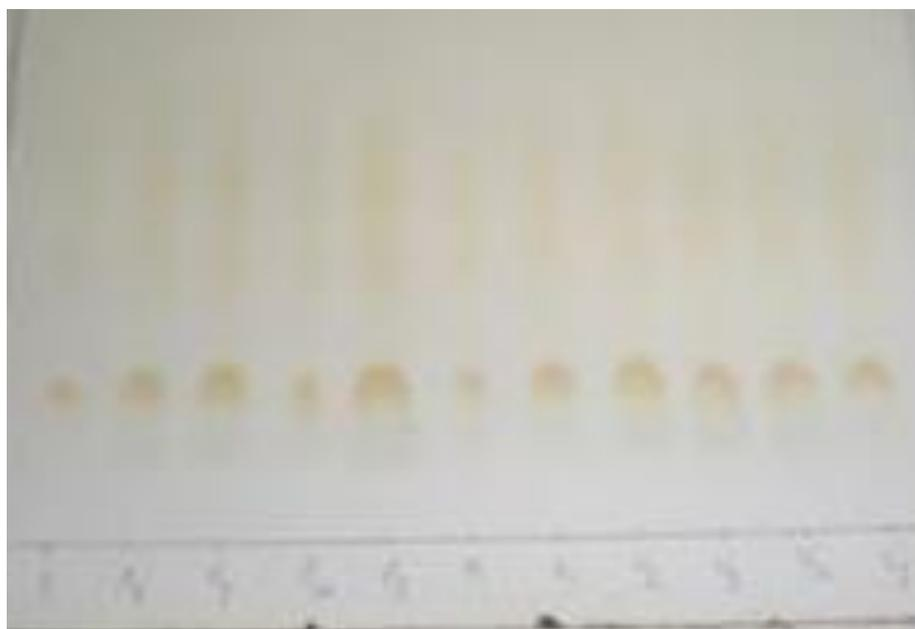
**Fig. 2. TLC plate photograph of Ampicillin samples**
