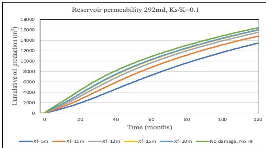
**Fig. 13. Effect of half-length on cumulative oil production**
