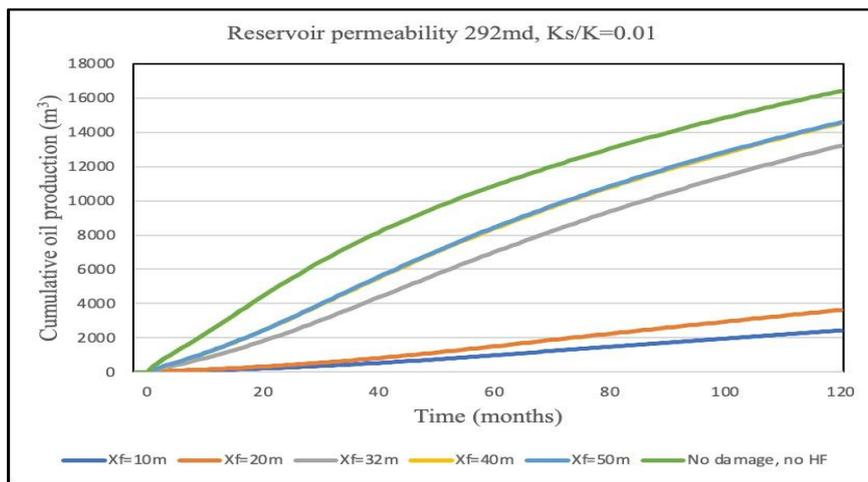
Fig. 12. Effect of half-length on cumulative oil production
