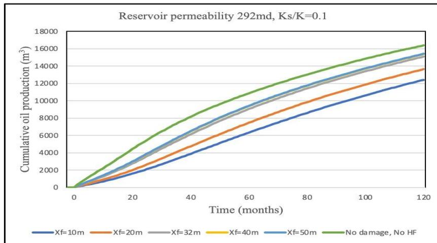
**Fig. 14. Effect of half-length on cumulative oil production**
