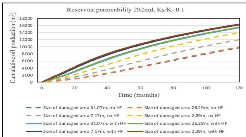
**Fig. 10. Effect of hydraulic fracturing on the size of damaged area (cumulative oil production)**
