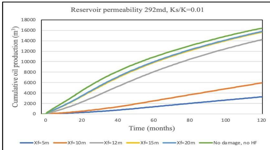
Fig. 11. Effect of half-length on cumulative oil production
