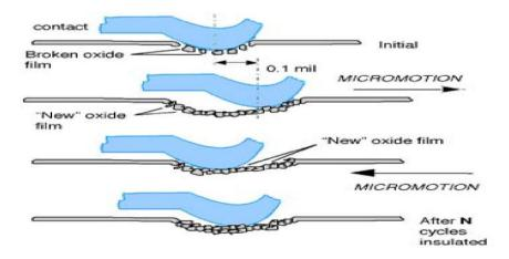
Fig. 2. Fretting Corrosion
