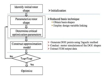
Fig. 2. Flowchart of design optimization process
