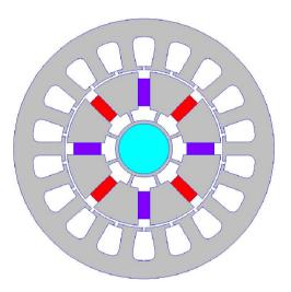
Fig. 1. Cross section of 8P18S IPM motor
