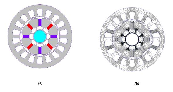
Fig. 6. Optimum resultant shape, (a) geometrical model, (b) finite element model
