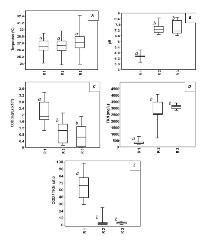
Fig. 2. Boxplots comparing A) temperature, B) pH, C) chemical oxygen demand (COD), D) total Kjeldahl nitrogen (TKN) and E) COD/TKN ratio in the three anaerobic digesters: R1 = effluent of cassava; R2 = effluent of cassava + urine; R3 = effluents of cassava + urine + cow manure. The different alphabets (a, b, c) indicate significant differences between the clusters based on the Mann-Whitney comparison test (p < 0.05).
