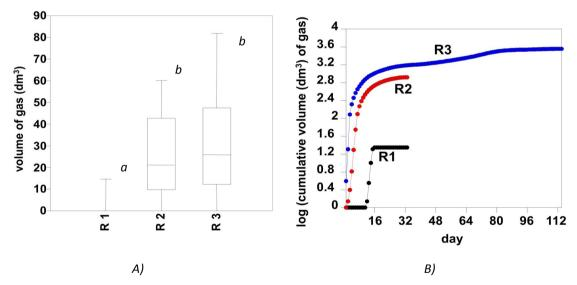
Fig. 3. A) Boxplots comparing biogas volume variation and B) cumulative volume of biogas in the three anaerobic digesters: R1 = effluent of cassava; R2 = effluent of cassava + urine; R3 = effluents of cassava + urine + cow manure. The different alphabets (a, b, c) indicate significant differences between the clusters based on the Mann-Whitney comparison test (p < 0.05).
