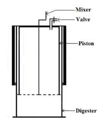
Fig. 1. Schema describing the experimental device
