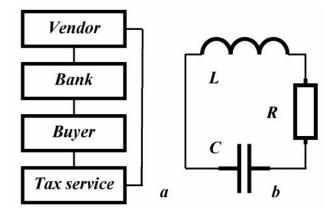
Fig. 2. Simplest oscillation links in economics and radio-electronics, where a damped oscillation process is observed
